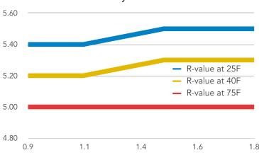
\*R-value means resistance to heat flow. The higher the R-value, the greater the insulating power. The R-value properties are based on 1.06 in thickness. Material density = pounds per cubic foot.
