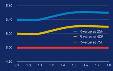
\*R-value means resistance to heat flow. The higher the R-value, the greater the insulating power. The R-value properties are based on 1-1/16 in thickness. Material density = pounds per cubic foot.
